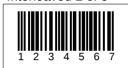
Interleaved 2 of 5 + CHECKSUM
